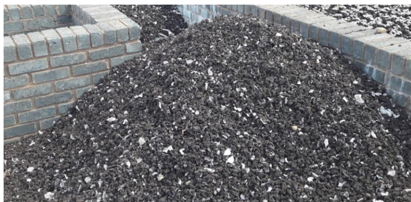
Figure 5.4: Unutilized dried sludge at NC-DM2-LM1-Plant1 that could be sold as manure after classification
