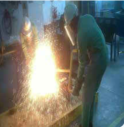
Students at the Gauteng Foundry Training Centre pour molten cast iron from the ladle into a sand mould
